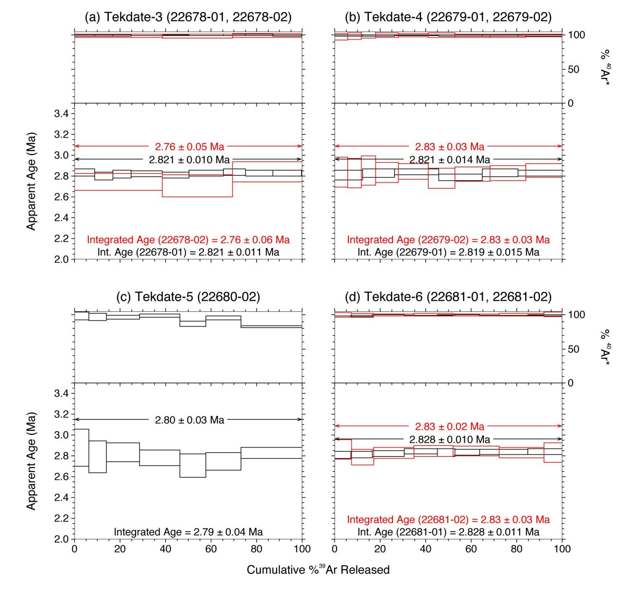
40Ar/39Ar incremental heating spectra for four glass samples attributed to the Healdsburgite strewn field. All spectra agree within uncertainty, and yield an overall mean age of 2.823+0.006 Ma (MSWD = 0.45, n=7)
